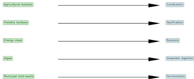
Fig.1. Biomass feedstock-to-energy conversion pathways including agricultural residues, forestry residues, energy crops, algae, and municipal solid waste (schematic flow diagram).
